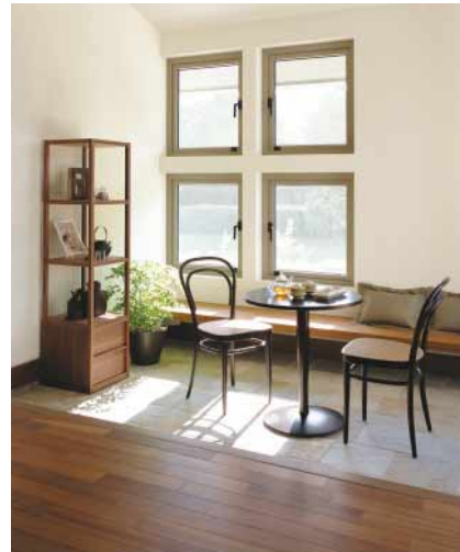
Sunlight warmth stored in the floor keeps this sunroom cozy warm in winter
